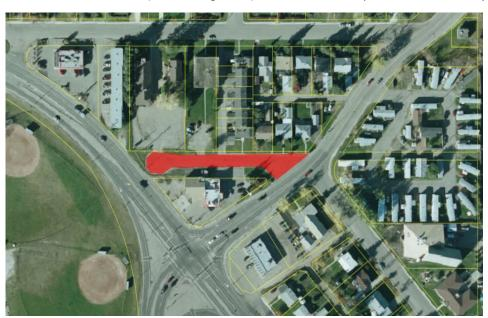
Remove existing asphalt, complete base repairs as needed, replace misc. sections of deteriorated concrete/missing from underground repairs, pave with 75mm asphaltic concrete. The underground utilities were replaced in 2015. This project will reinstate the existing road surface and concrete sections
