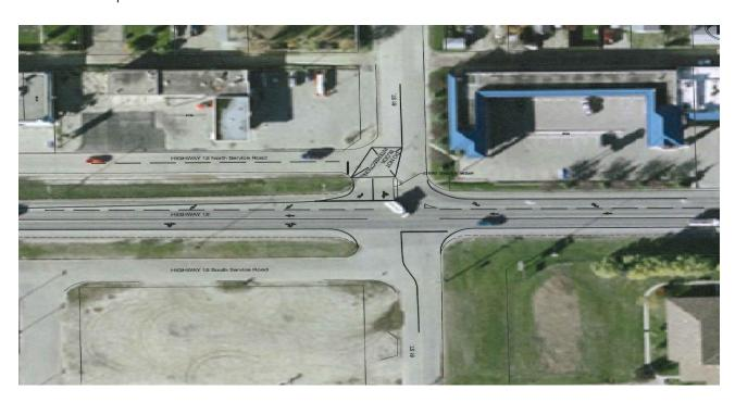
The second proposal includes the intersection at 67 Street (Tim Horton's/McDonalds) complete with signalized traffic lights with a slight widening of the north side of the highway to accommodate changes to lane configuration. The master plan includes an option for overlay pavement of the intersection, which we feel would be ideal for establishing paint lines for a total intersection improvement cost of \$700,000.
