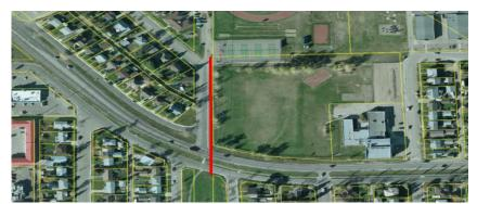
confirmed the culvert is completely rotted and in need of replacement. This storm main is a collector main and a critical piece of infrastructure to prevent flooding. Not replacing the main has the potential for liability and insurance claims if a collapse happened and storm water couldn't flow.
