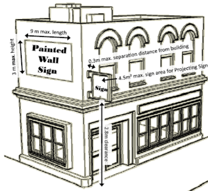
Figure 72-1: Painted Wall Signs and Projecting Signs
